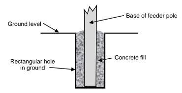
• Look back at the depth into the ground to which the pole must sink. The hole for the concrete fill should be at *least as deep as the depth of the pole below the ground*, and *at least a quarter (0.25)* of this distance wide.
